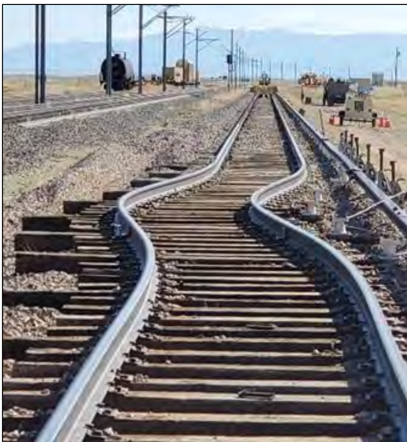
Track Buckle from 2022 MxV Rail/BNSF Test
