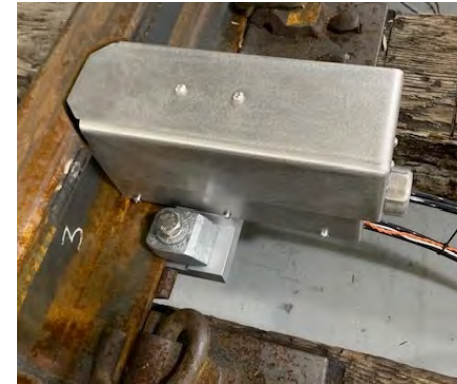
EMAT sensor assembly with actuator
