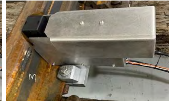
EMAT sensor assembly with actuator
